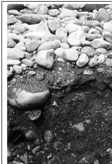
Fig. 1. Bed sediment of the River Wharfe, U.K., showing a pronounced surface armor. Image courtesy D. Powell.
