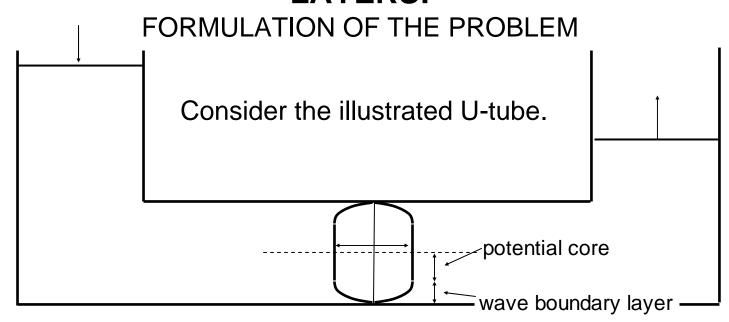
$$\frac{\partial \overline{u}}{\partial t} + \overline{u} \frac{\partial \overline{u}'}{\partial x} + \overline{w} \frac{\partial \overline{u}'}{\partial z} = -\frac{1}{\rho} \frac{dp_w}{dx} + \frac{1}{\rho} \frac{\partial \tau}{\partial z} - g \frac{\partial \eta}{\partial x}$$
