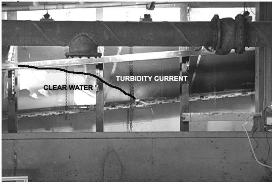
Figure 4b. A turbidity current with an upstream temperature difference  $\Delta T$  of  $62^\circ$  tends to billow upward as it propagates downslope (SERIES 2 run a). The flow is from left to right. The black line was inserted to illustrate the approximate boundary between clear water and sediment-laden water. Note that although the bed slopes to the left, the interface between the sediment-laden and clear water slopes to the right.
